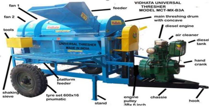
Figure 1: The Vidhataa multi-functional thresher
